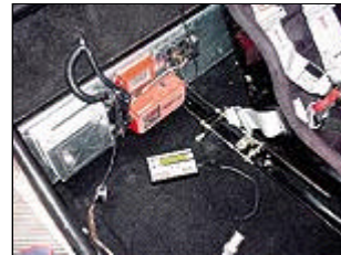
The ignition electronics are located behind the passenger seat.
