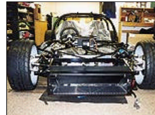
The cooling system is immense. The brass-and-copper-constructed radiator with twin fans sits at the front of the car. The coolant is routed to the Chevy pump situated amidship by pre-formed aluminium tubes and silicon hoses. This standard system has been designed to cool engines producing up to 550 hp.
