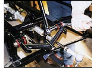
TIG-welded wishbones are mounted on the chassis using urethane bushes. A fully rose-jointed option is available, but for road and most track use the standard setup is formidable.
