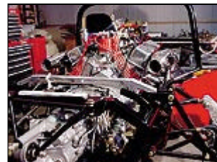
The removable rear crossmember modification makes installing the engine/transaxle a snap.
