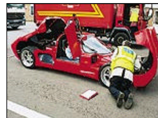
Here the car is going through its SVA test. This is the UK procedure for registering a car for road use. After a four-hour inspection, it passes with flying colors and is now nestled in
