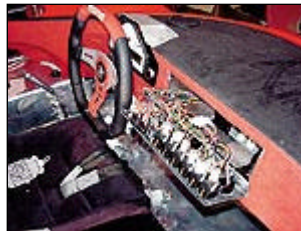
Rosen also customized his own dash. The swing-down control panel makes access to the switches a snap.
