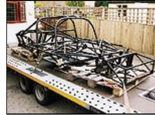
The GTR triangulated spaceframe chassis was delivered. Integral roll-cage is welded to main frame.
