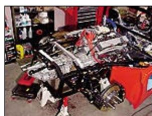
A Porsche G50 transaxle transmits the estimated 500 hp that Rosen's '72 GM 350ci engine will produce.
