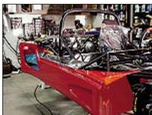
With most of the mechanicals in place, the body sidepods are installed next.
