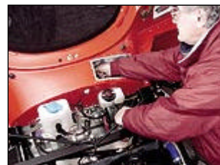
Much-needed access is gained through a custom hatch fabricated by Rosen.
