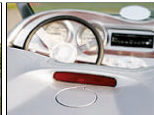
Burchett made the custom brake lights and installed a third brake light right behind the edge of the cockpit.
