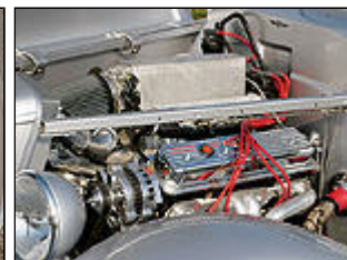
The powerplant for the lil' roadster is a 350/350 GM Ram Jet crate motor, backed to a TH350 transmission. Internally left stock, the exterior utilizes extra performance goodies such as an Edelbrock water pump, Powermaster alternator, a K&N air filter, headers from Sanderson, and Flowmaster mufflers.
