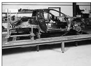
First the Fiero was stripped of all nonessential items, such as the running gear, rear suspension, rear brakes, body panels, interior, and bumpers. The frame was bolted to the table with metal jigs fabricated by Terry Fisher. The jigs kept the frame from moving as it was cut apart and welded. The adjustable legs on the table allow it to be precisely leveled to keep everything square. The frame was checked to make sure it was square. Note: This is also how racing cars are built.
